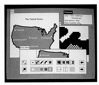
The 4404's 640x480 display functions as a window into a 1024x1024 bit-map memory, with smooth panning whenever the cursor reaches a physical display edge. Users also have the ability to point with the mouse and integral joydisk.
