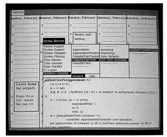
The 4404 facilitates quick, efficient prototyping. Pageon-demand memory management provides a large, 8-Mbyte virtual memory address space that permits development of complex programs without segmentation or overlays.
