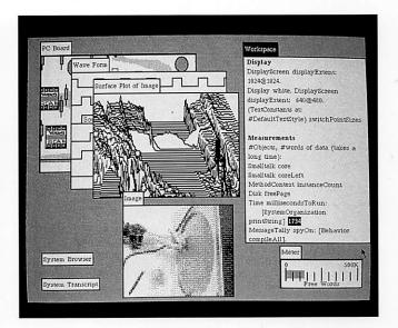
With its proprietary Smalltalk-80 implementation, graphics performance on the 4404 makes on-screen animation possible. The Smalltalk-80 package offers advantages of a highly integrated programming environment and object-oriented language with an excellent user interface.
